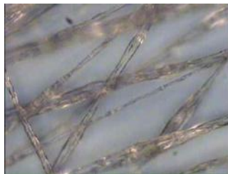
Figure 2: Electrospun Cloisite 20A + PMMA fibers under 50x magnification
