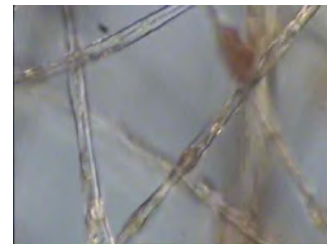
Figure 3: Electrospun nanocomposite + PMMA fibers under 50x magnification
