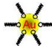
Figure 1: Gold nanoparticles with attached thiol chains.
