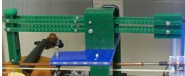
Figure 1: The pressure system used to accurately measure the vertical force of the bow on the string.
