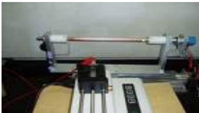
Fig. 1 Electrospinning fibers on a rotating mandrel
