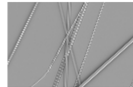
Figure 1 3000x magnification of 35%wt P4VP fibers
