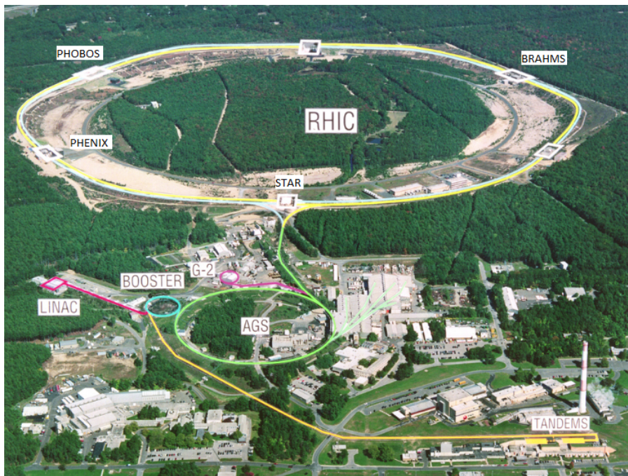
Figure 2.1: Aerial view of RHIC. The location of the four experiments are labeled along the ring. The tandems, AGS and other components which aid in the production and acceleration of the beams are also included and marked in the image.
