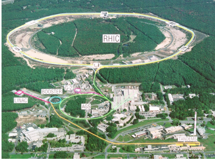
Figure 2.1: An Aerial photograph of the RHIC Complex with beam lines indicated.
